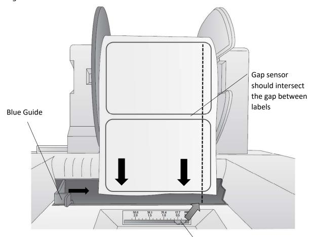
**Note** the position of the label sensor. Slide the sensor position indicator so that it intersects with the gaps between your labels. For most label stock you will not need to move this. Gap Sensor Position Indicator from right edge of media. The position indicator corresponds to the ruler NOT the installed label stock.
