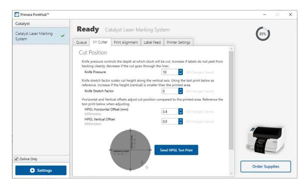
**Cut Offsets** If your cut does not line up with your printed image, you can adjust it using the **Horizontal Offset** and **Vertical Offset** settings. Press the Send Test Print to help you determine which direction to move the offsets or refer to the image below.
