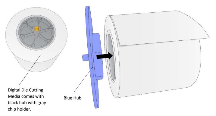
3. Set the roll in place so that the blue pin sits in the notch on the roll holder.
