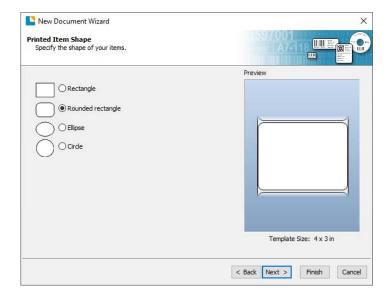
8. Set the template size to match labels installed in the Printer. Change the Template Size to User Defined Size to gain access to width and height. Click "Next".
