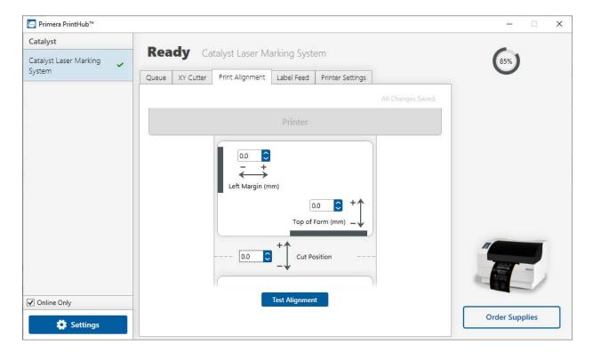
Click on Test Alignment to print the alignment shown to the right. Look at the print to determine how much white space is visible on the edges. The black lines should print right on the leading edge and left edge. In this example the Top of Form needs approximately - 10.
