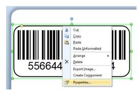
3. Adjust the Width, Height, Corner Type and Corner Size (Radius). A typical corner radius is .125".
