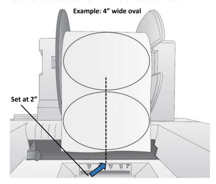
**Important Note**: You must adjust the stock sensor <u>before</u> loading nonstandard label stock.
