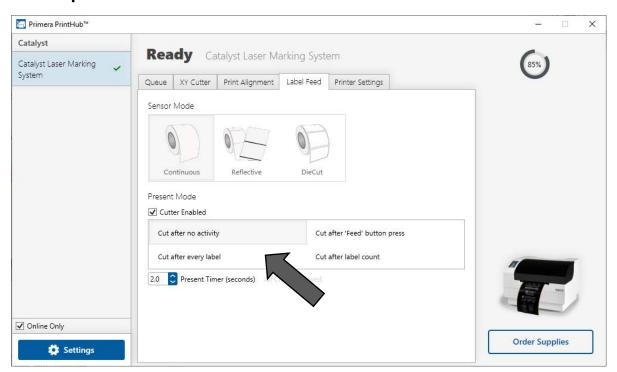
**Cut after button press.** This setting will cut after you press the Load/Feed button on the Printer. This can be used after one label or an entire job. This feature is useful if you will not be present at the end of the print to catch the cut label.
