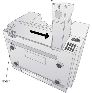
4. Install the roll guide by attaching the hooked end on the rail. The bottom of the holder will fit in the notch on the Printer.
