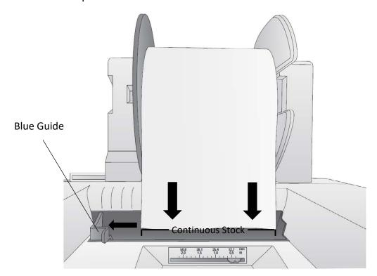
7. **Die-Cut Media.** Guide the leading edge of the roll into the feed area. Move the blue guide so that it touches the label stock.
